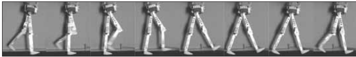
RunBot's program mimics the way neurons control reflexes in humans and other animals.
