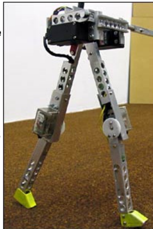
RunBot can adjust its speed when going up or down a slope
